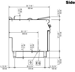
EQ = Equipotential screwG = Gas connection
